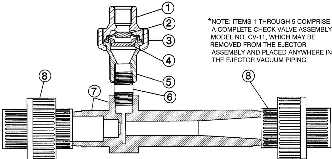
\*NOTE: ITEMS 1 THROUGH 5 COMPRISE A COMPLETE CHECK VALVE ASSEMBLY MODEL NO. CV-11, WHICH MAY BE REMOVED FROM THE EJECTOR ASSEMBLY AND PLACED ANYWHERE IN THE EJECTOR VACUUM PIPING.
